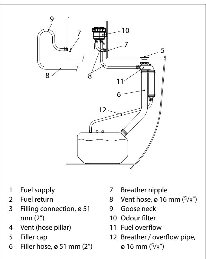
Fit all hose connections using 2 stainless steel hose clamps!
