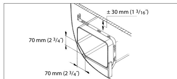
Make sure the tank has a sufficiently secure foundation on which to install it and secure it properly. **The dimensions of the tank will increase a little when it is filled.** Take this into account when fixing the tank.
