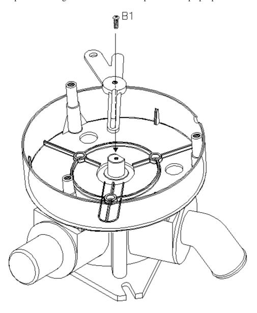
Step 5. Check carefully, the blue hand and rotary arm be in same direction before going to Step 6.
