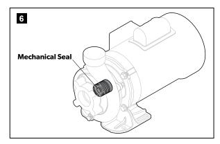
**NOTICE** DAMAGE HAZARD: When replacing mechanical pump seals, keep the seal surfaces clean. Do **not** touch seals or related surfaces with bare hands to prevent oil from transferring to the surfaces. Failure to follow this instruction could lead to excess leakage and cause property damage.
