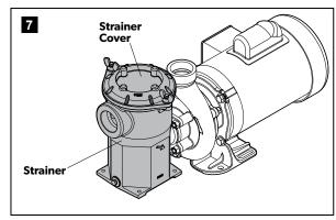
The strainer basket on the PR115R needs to cleaned periodically to ensure the proper flow rate to attached water-cooled equipment, and to reduce stress on the pump:
