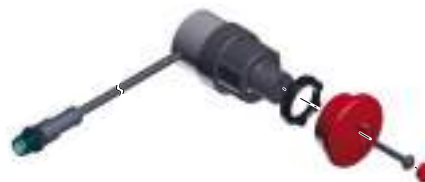
Fig. 49: Emergency Off switch installation drawing
